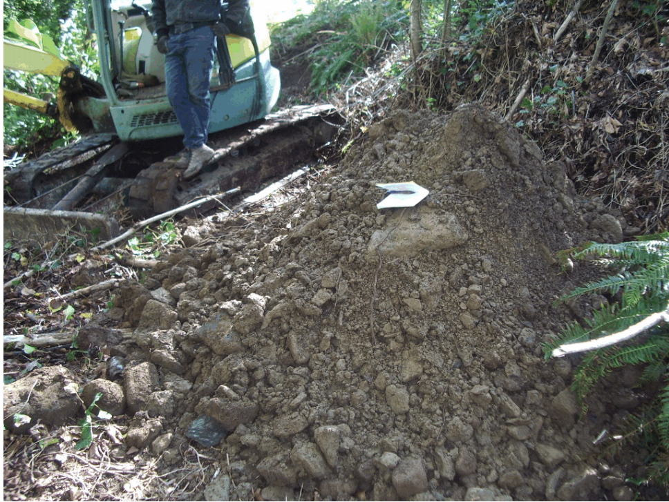
Photo 1 - Spoils from test pit TP-1. Note the rocky nature of the excavated materials.
