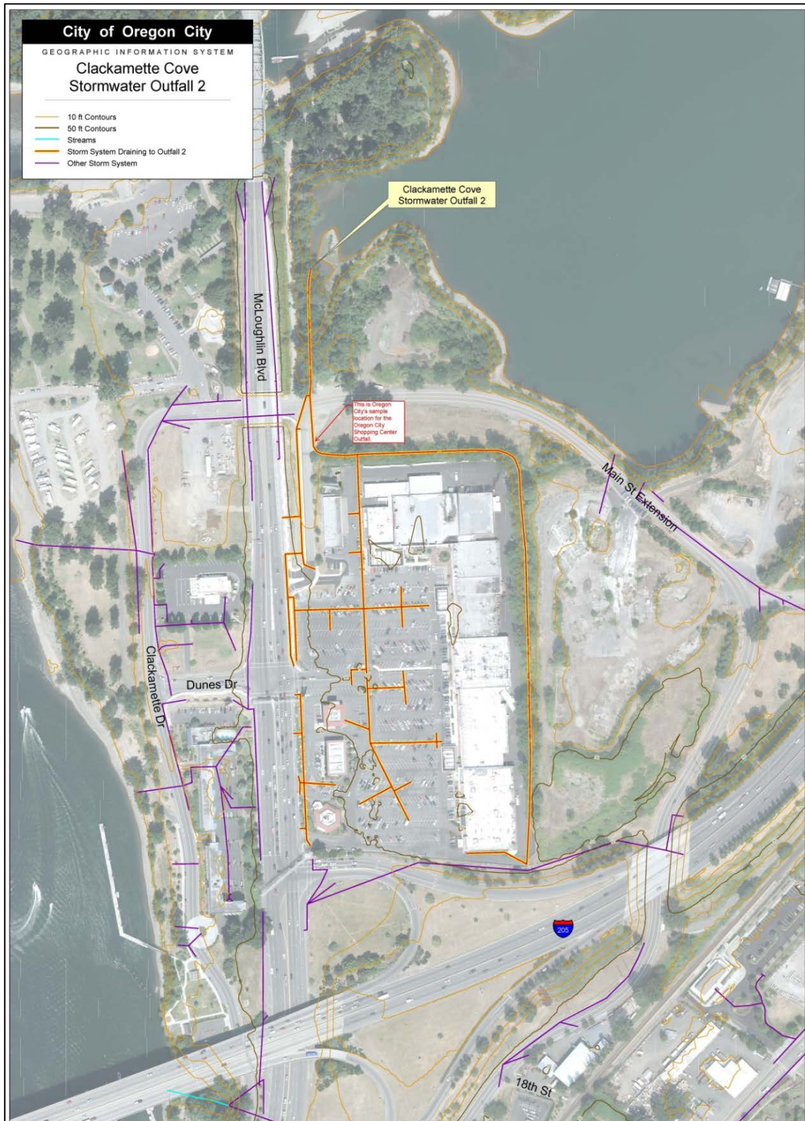
Figure 11. Clackamette Cove stormwater outfall 2 and associated conveyance system. Water quality monitoring samples are collected at a site near the shopping center. Graphic courtesy of the City of Oregon City.
