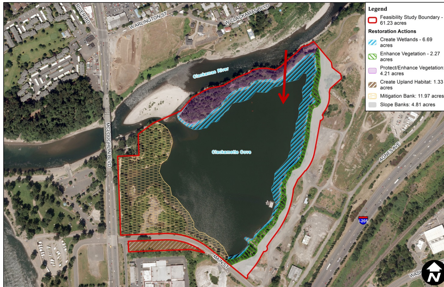
Figure 14. A conceptual habitat and water quality enhancement design for Clackamette Cove that integrates improved connectivity to the Clackamas River (red arrow) with habitat restoration actions and a habitat mitigation bank.
