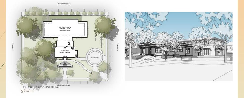
A 2 story option allows the playground to stay in its current spot. This option uses the original Carnegie entrance as the main entrance. The stairs are extended out, and a ramp is put in for ADA compliance.
