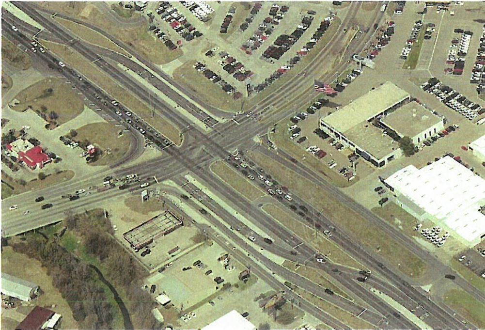
Exhibit 1-4. Four-legged DLT intersection with major street displaced lefts and channelized right turns (Baton Rouge, LA). (1)
