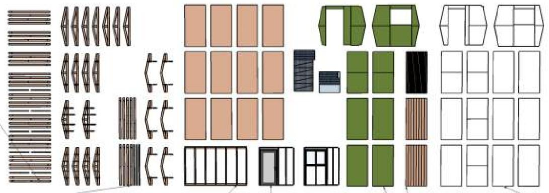
Total Material needed for Primary Truss Assembly (17 Trusses Total): (100) SDWC Screws (varied lengths) (288) Screws (34) 8' long 2x4's (5) 8' long 2x2's
