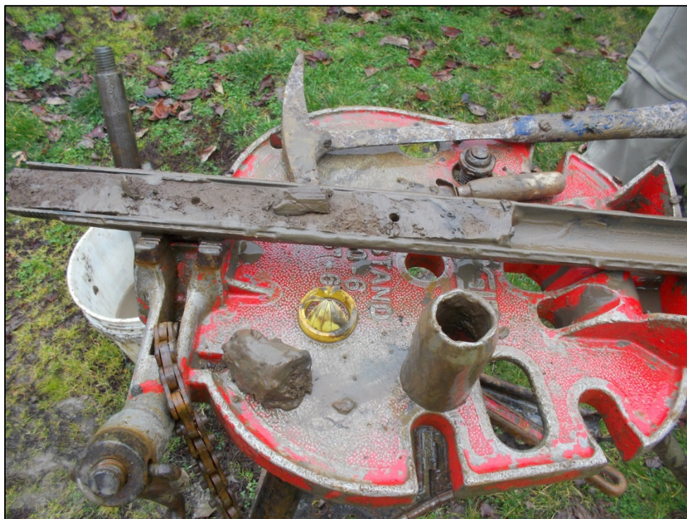
Figure 4. Boring B1. Opened 1.5-inch-diameter split spoon sample showing Stratum I and Stratum II interface (Fill/ACb horizon interface), at 2.4 m (8 feet) below ground surface. Interface roughly at hammer head, with fill (right/upcore) and ACb (left/downcore).
