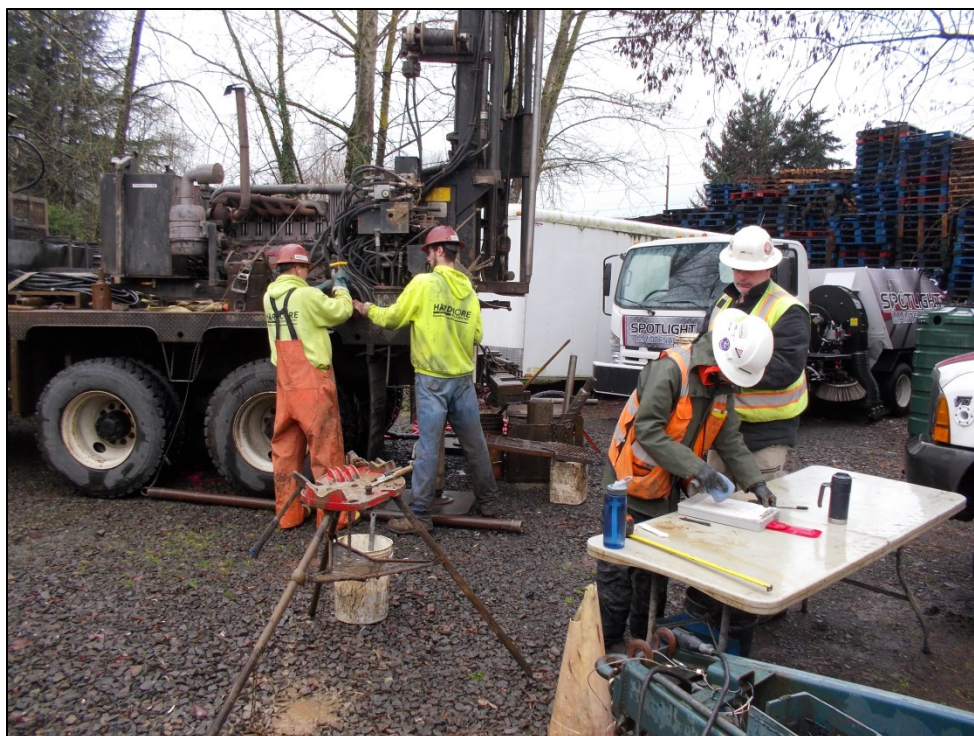
Figure 3. Hardcore Drilling CME 75 drill rig and crew at boring B4 (left). GeoDesign Inc and SWCA logging core samples (right). View northwest.
