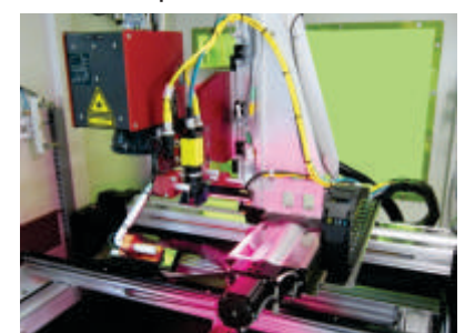
XYZ motion & vision for alignment & verification
