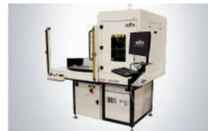
Rotary table system, 4-positions; 3 for load/unload/inspect and 1 for marking
