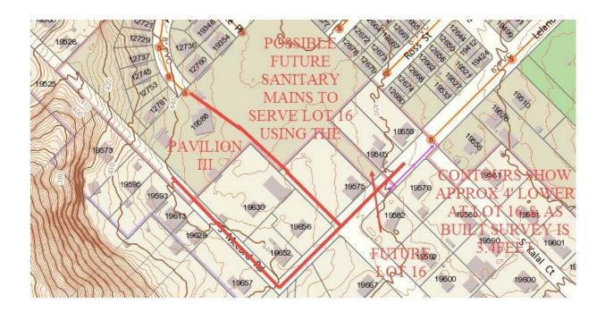
The as built elevation of the manhole at Leland and Kala Court has a rim of 449.75 with IE in of 437.47. The ground elevation in Leland Road slopes westerly with an elevation opposite future lot 16 of 446.36. The existing ground continues to slope westerly. Future mains from McCord or from Pavilion III would serve this area.
