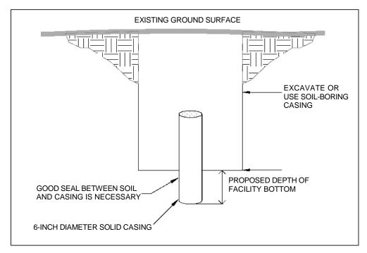
Figure D-1. Encased falling head procedure
