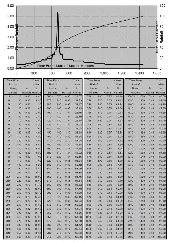
Figure H-1. NRCS 24-Hour Type 1A Hyetograph
