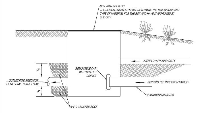
Planter, Rain Garden, Swale Flow Control Structure Figure C-10
