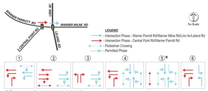
★ Phase necessary if a pedestrian crossing is desired for the east and west legs of the Central Point/Warner Parrott Rd. intersection.
