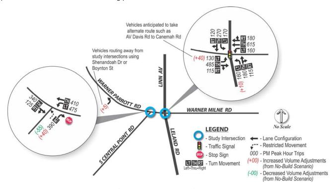
Figure 4: 2035 Intersection Volumes for Alt 2: Unsignalized Left-Turn Restriction without Signalized U-Turn
