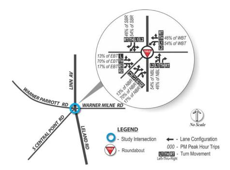
Figure 7: Intersection Volume Adjustments for Alt. 5: Five-Leg Roundabout
