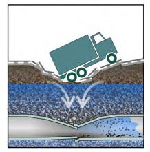
Figure G-8. Structural failure mechanism caused by infiltration at joints
