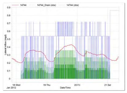
Figure 10. Pease Road Pumping Station wet well inflow calibration, January 19, 2012 event red = simulated, blue = estimated (pump run), green = estimated (wet well drain)
