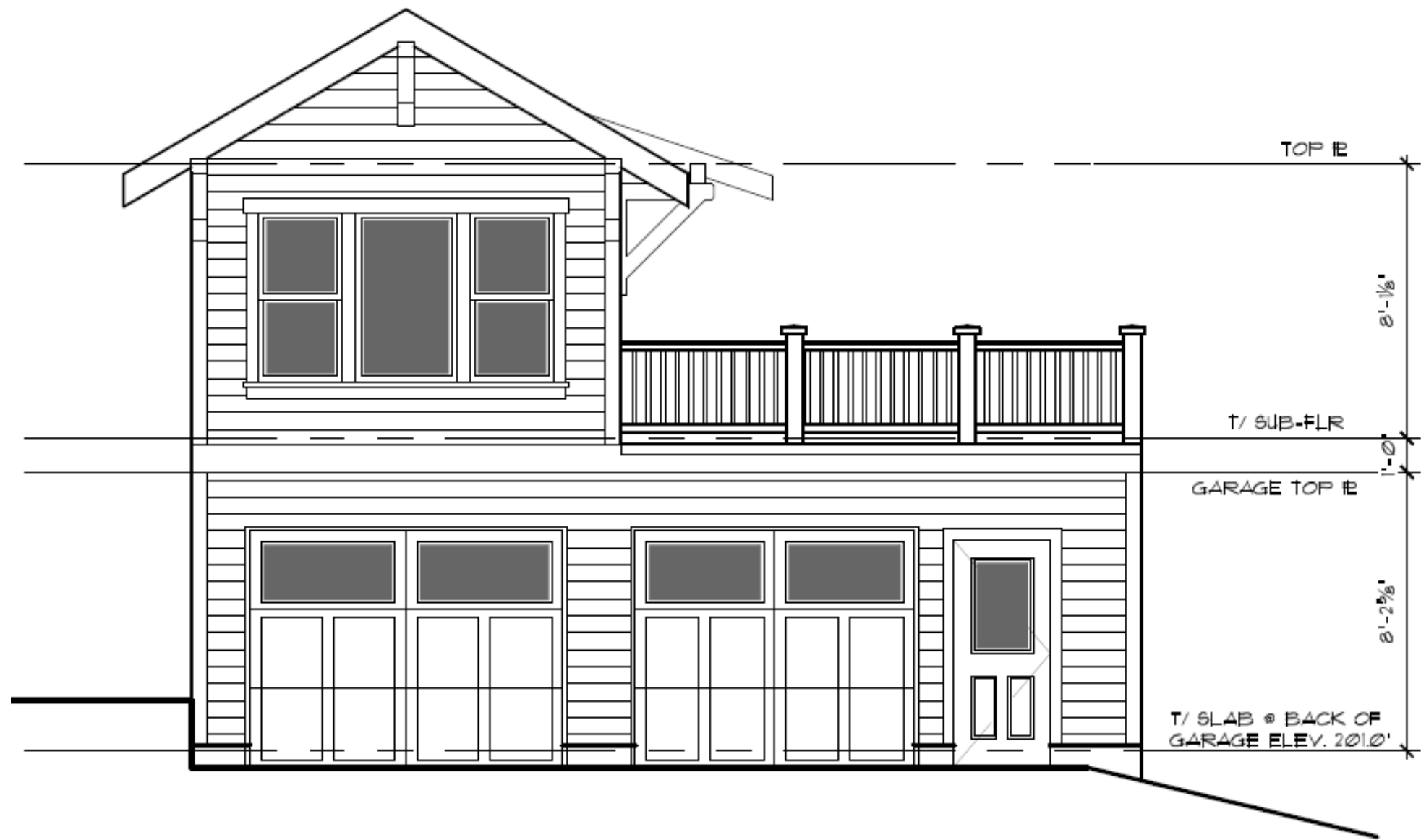
LEFT SIDE ELEVATION - GARAGE
